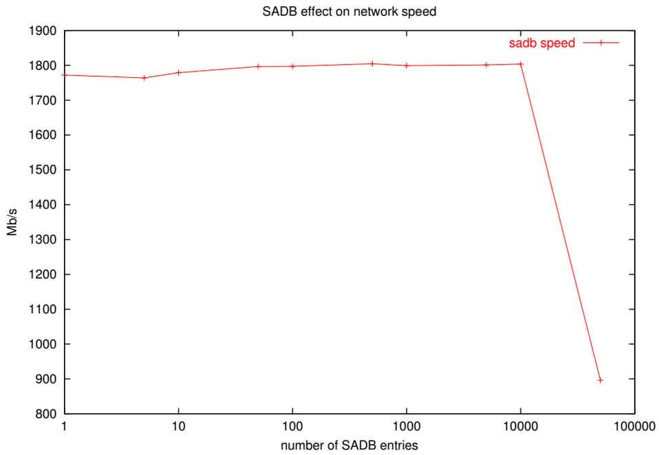
Figure 8: sadb processing and its effect on network speed
