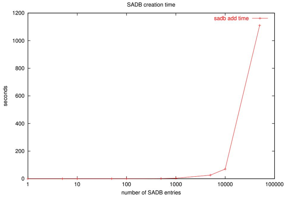
Figure 7: sadb insertion processing speed
