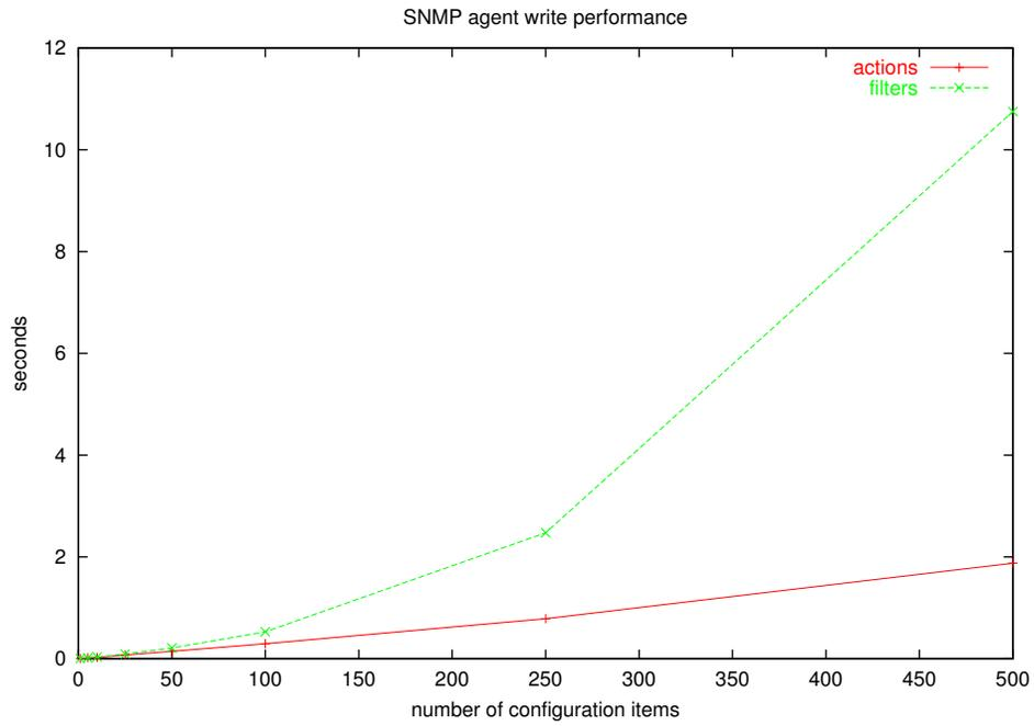
Figure 10: Time required to perform configurations via SNMP
