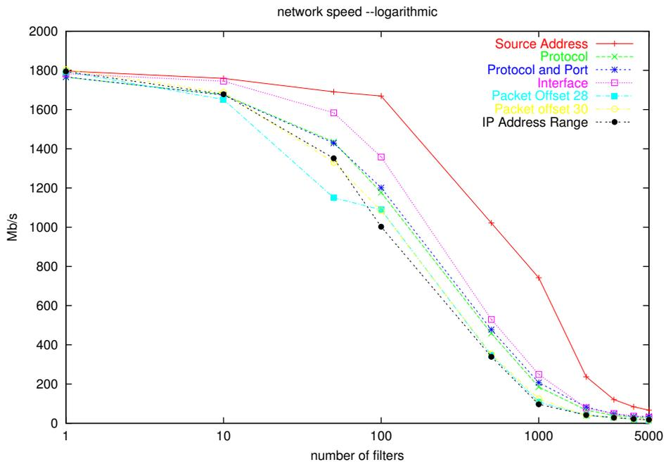
Figure 6: Filter processing and its effect on network speed – logarithmic scale
