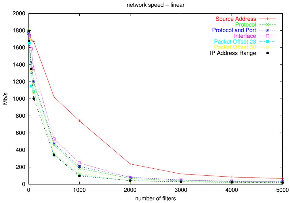
Figure 5: Filter processing and its effect on network speed – linear scale
